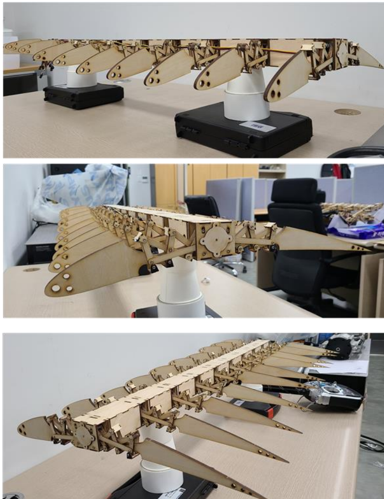
Fig. 42 Variable Camber Morphing Wing deformed as a twist morphing wing
