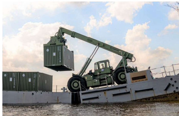
Figure 5- Rough Terrain Cargo Handler (RTCH) lifting a standard ISO container
