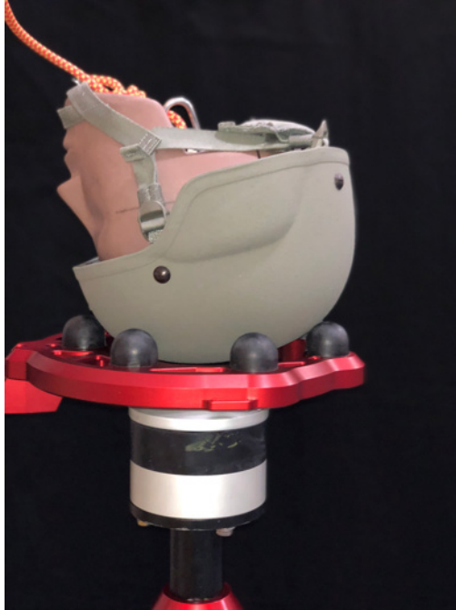
Fig. A-9 Basket drop configuration with male 50% Hybrid III head and neck ATD in pose for the crown impact location
