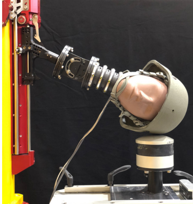
Fig. A-7 Monorail with neck configuration with male 50% Hybrid III head and neck ATD in pose for a side impact location
