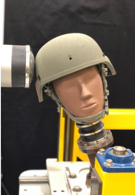
Fig. A-3 Pneumatic ram machine configuration with male 50% Hybrid III head and neck ATD in pose for a side impact location
