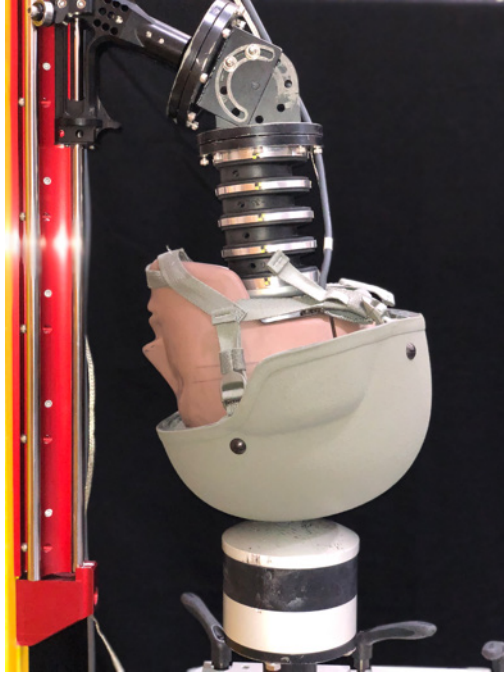
Fig. A-5 Monorail with neck configuration with male 50% Hybrid III head and neck ATD in pose for the crown impact location
