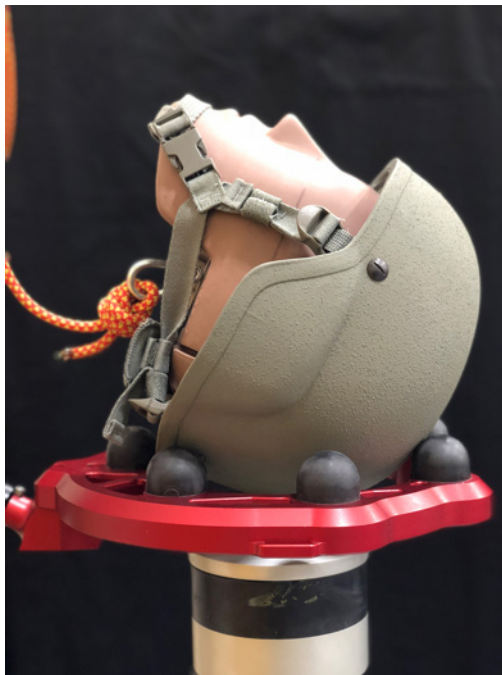
Fig. A-10 Basket drop configuration with male 50% Hybrid III head and neck ATD in pose for the rear impact location
