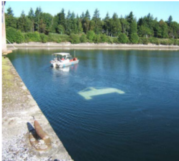
Figure 4-3. Geophysical Prove-Out of Marine Magnetometer Survey, Ostrich Bay, WA. A pontoon boat towed the sensor platform, which is submerged 7 ft below the surface.
