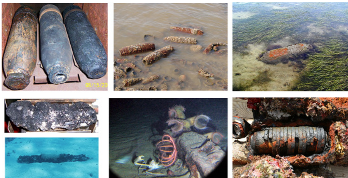
Figure 2-1. Examples of munitions in U.S. waters. Note variable condition and degree of encrustation, which may affect dissolution of MC to the surrounding environment.
