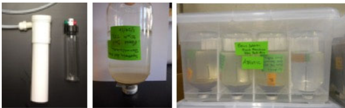
Figure 4. Photos of 40 mL glass vials & 160 mL glass bottles used in batch studies, with double containment approaches to maintain anaerobic conditions and/or minimize volatilization losses.
