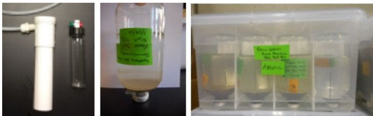
Figure 3.4. Photos showing 40 mL glass vials and 160 mL glass bottles used in batch studies, along with double containment approaches to maintain anaerobic conditions and/or minimize volatilization losses.
