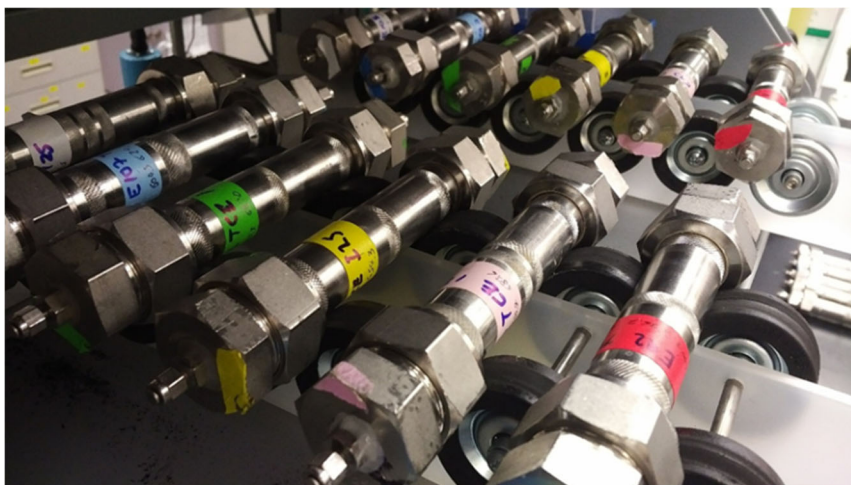
Figure 4. 5. Rolling Tube Reactors (RTR) reactors used for the kinetic studies. Here they are shown on the roller system that rotated them at ~10 revolutions per minute
