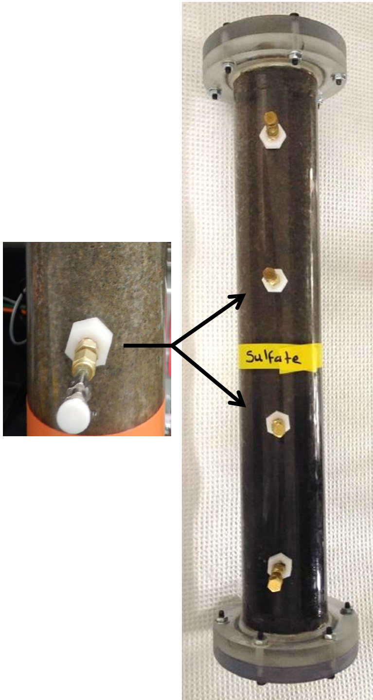
Figure 4. 2. Photographs of one of the soil columns used for this project. The insert shows detail of the sample port construction, which is further described in the text.
