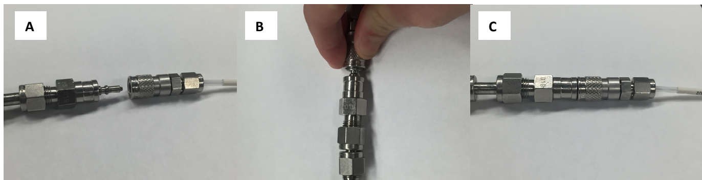
Figure 2. (a) Swagelok female quick-connect (on the Aura (right)) and the Swagelok male quick-connect (on the canister (left)); (b) Swagelok being pulled open for connection; (c) Connected Aura flow controller to a canister.
