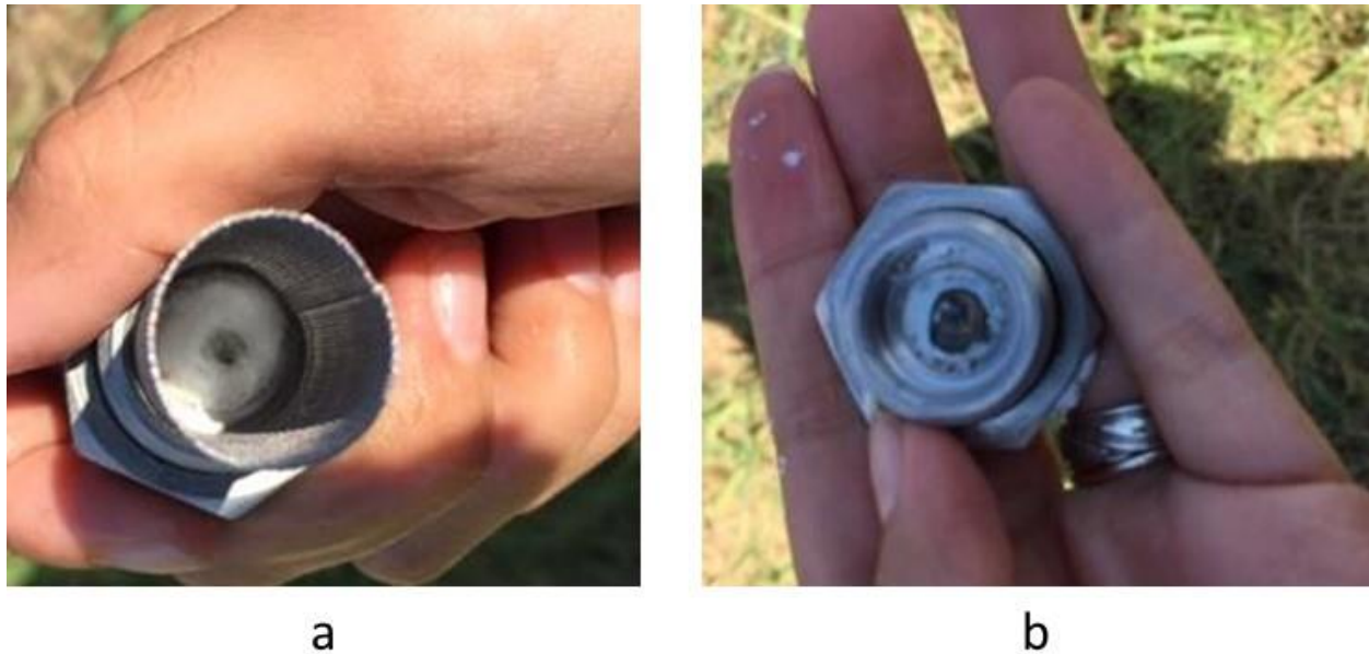
Figure C-3. White Paste Material Present on Set Plug: (a) On Strainer Screen and (b) On Housing
