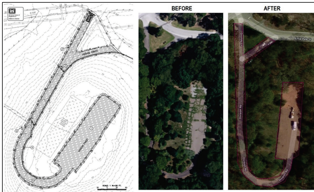
Figure 6-6. Division Hill pavement removal depicted on construction plan documents and before and after satellite imagery.
