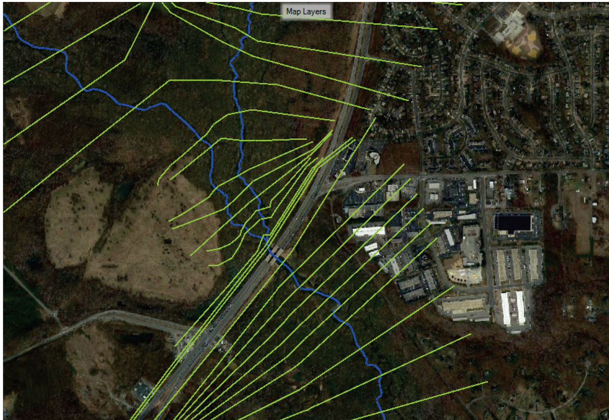
Figure 5-3. Sample Google image with cross-section cutlines.
