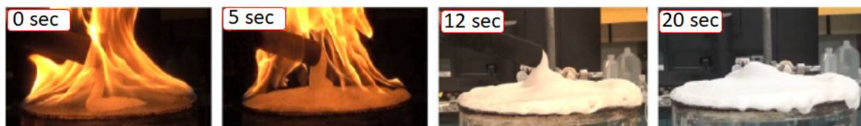
Figure 90 Ref AFFF foam flowing onto heptane pool fire at 1500 mL/min which extinguished the fire in just 12 seconds at this rate.
