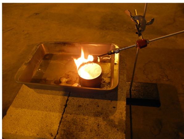
Figure 27 Small-scale pool fire testing apparatus for the new surfactants, gasoline test fuel in 3.25" pan.
