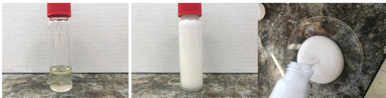
Figure 78 (left) APS added onto water solution of AA (1:1 ratio); (center) mixture then vigorously shaken; (right) freshly made APS/AA had strong foamability.
