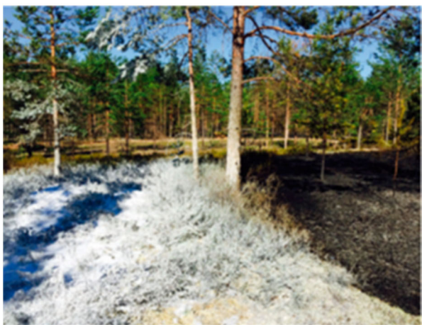
Figure 16 Vinogradov et al. demonstrated fire fighting with a foam that created massive quantities of silica gel to cover a fire. In brief, a solution of sodium silicate is neutralized with acetic acid creating an amorphous silica blanket; enlarged photo of the resulting silica product.
