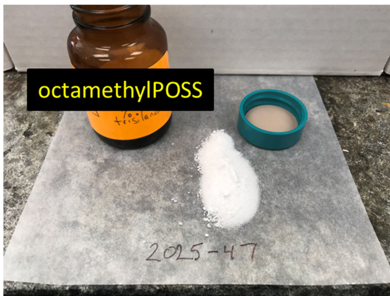
Figure 40 OctamethylPOSS product from cyclization of methyltriethoxysilane.
