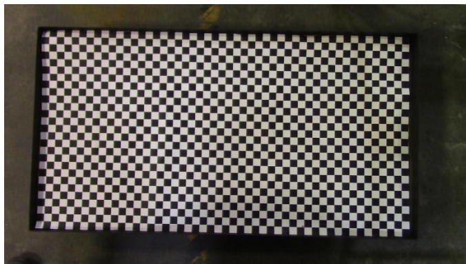
Figure 7– 20 x 20 mm grid used to calibrate video camera area analysis
