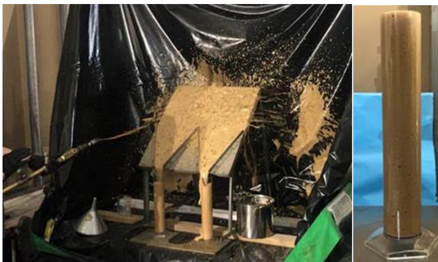
Figure 4. Foam drainage and expansion ratio testing at Jensen Hughes. Performed with 3%(w/v sPI (PMDA-BDSA-NA), 0.15%(w/v) sodium dodecyl sulfate (SDS) surfactant in water.
