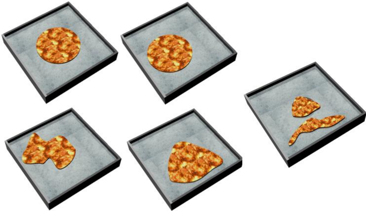
Figure 16 – Burnback test – examples of 25% pool area
