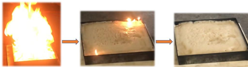
Figure 10. Progression of extinguishment for Generation 6, from pre-burn to suppression/control to extinguishment
