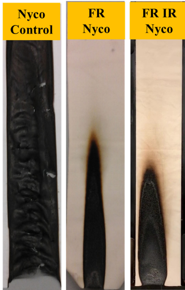
Figure 8: Post VFT images of Nyco control FR Nyco and FR IR Nyco
