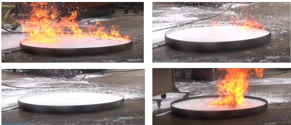
Figure 6. 28ft 2 MIL-PRF 24385F fire tests showing 90%, 99% control, extinguishment and burnback.
