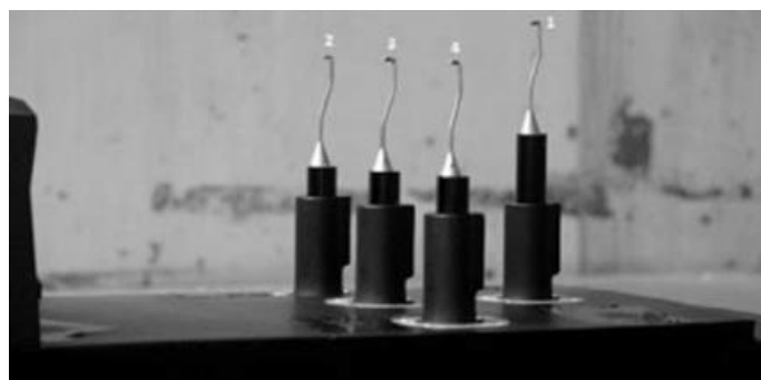
(b) probes used to measure airwake velocities
