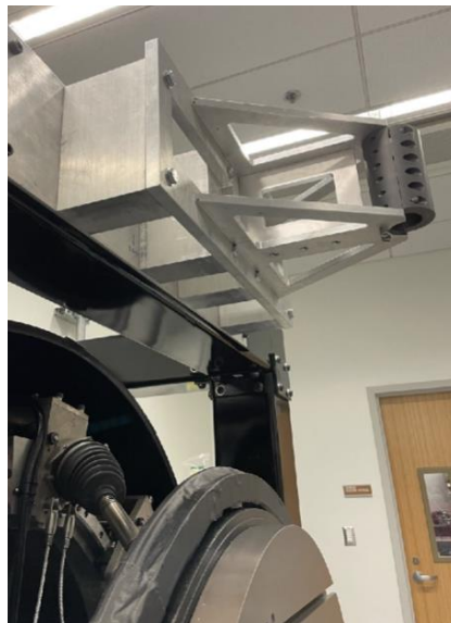
Figure 4: The prosthetic foot tibial mount shown above attached to the RGS which will be used to attach commercial prosthetic feet during mechanical testing.
