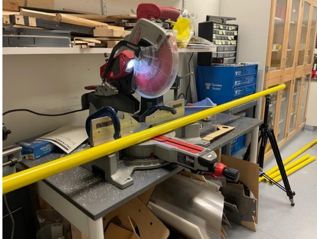
Figure 5: The motion capture camera mounting frame design was fabricated in-house to mount cameras for prosthetic foot mechanical testing data collection (frame members shown above in yellow).
