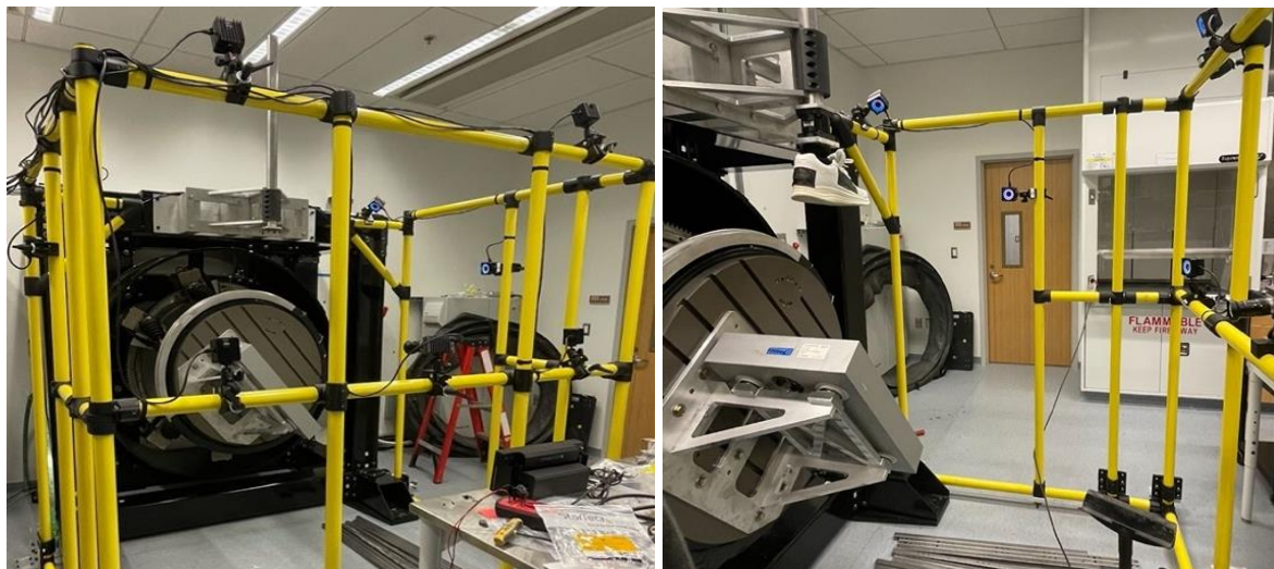
Figure 7: The OptiTrack cameras were installed and configured around the RGS to capture kinematic data as part of prosthetic foot mechanical testing.
