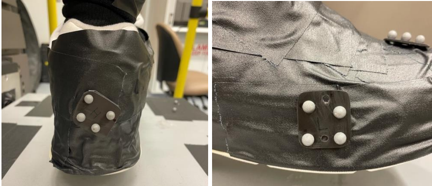
Figure 11: Rigid clusters of reflective markers on the heel (left) and forefoot (right) of a prosthetic foot and shoe are shown. These markers are detected by the 8-camera Optitrack motion capture system to track kinematics during mechanical testing.
