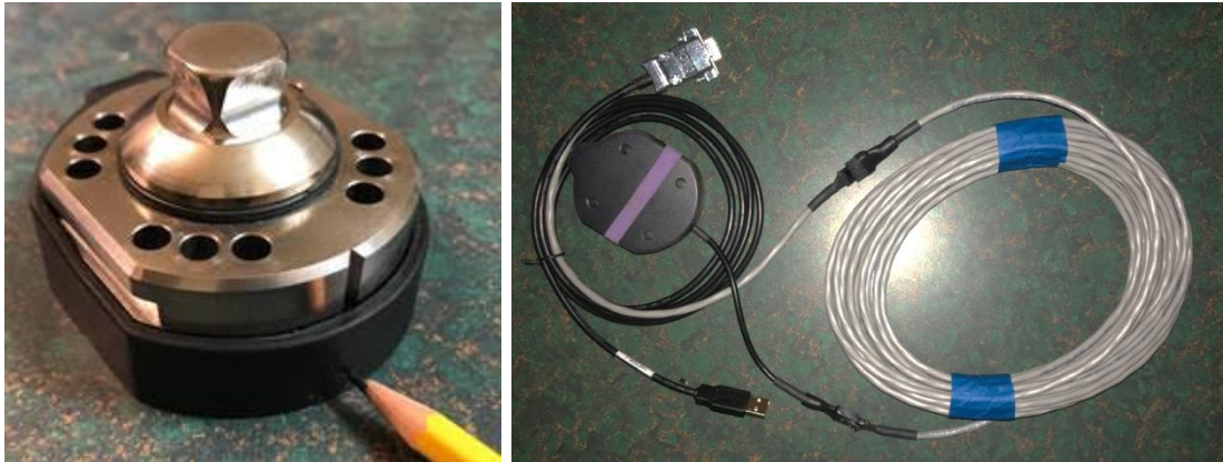
Figure 1: The Europa+ sensor as viewed from top (left) showing prosthetic pyramid adapter, and from the bottom (right) with custom wiring to interface with multi-axial prosthetic foot emulator equipment for testing to achieve equipment readiness for human subjects data collection.
