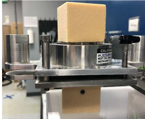
Figure 12. Resorption assembly for the dynamic prototype device showing the upper synthetic bone block, load cell, custom resorption stage, and lower synthetic bone block.
