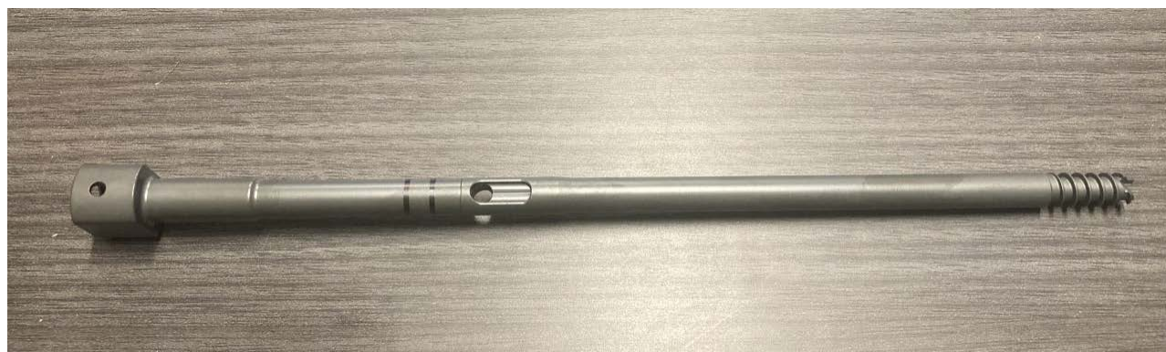
Figure 16. Fully assembled device with nail guide on left side and dynamic prototype device on right side.
