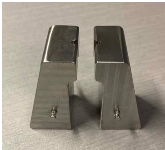
Figure 11. Machined set of grips for torsion testing.
