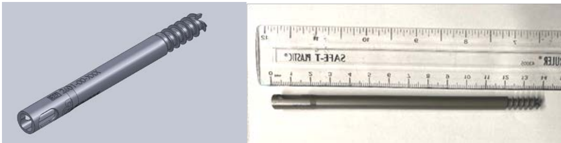
Figure 1. (left) CAD model of final dynamic prototype device. (right) Manufactured dynamic prototype device.
