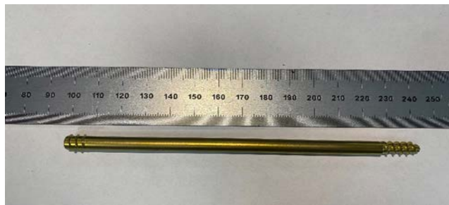
Figure 2. Static predicate device for pull-out testing.
