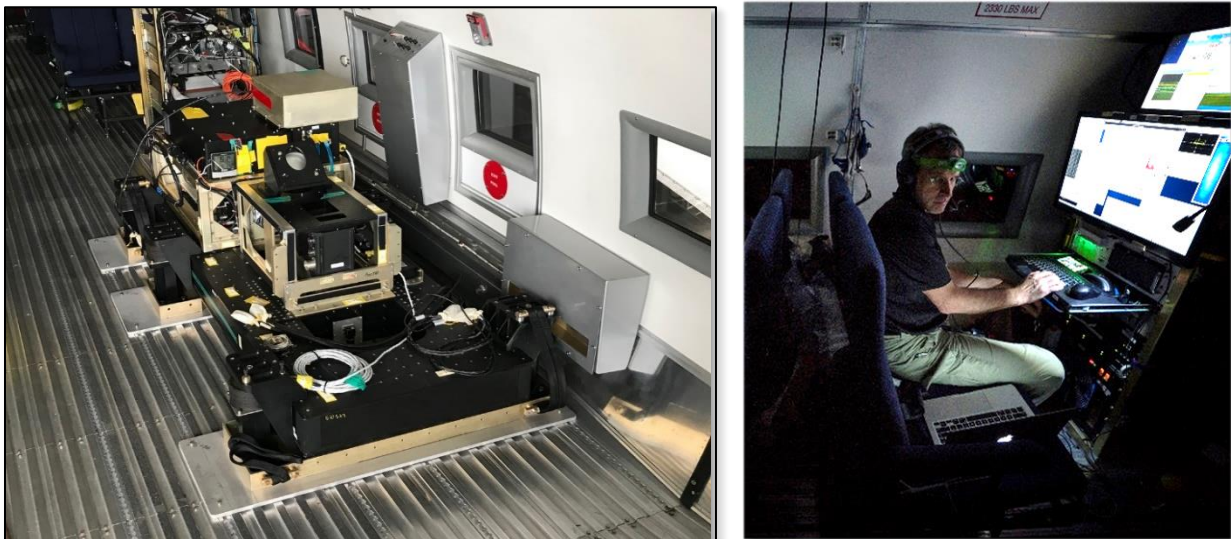
Figure 3. The AOSTB sensor instrument on board the BT-67 aircraft. 3DEO LIDAR engineers played an extensive role in flight planning, mission command, and sensor operation throughout the data collection campaign.
