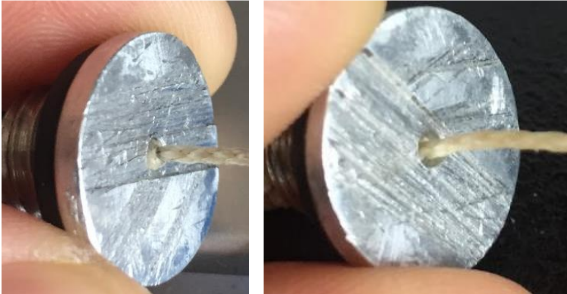
Fig. 8. Knot Slippage. Left image: Knot slipping through the hole that holds the tether. Right image: Knot sitting above hole and not pulling out.
