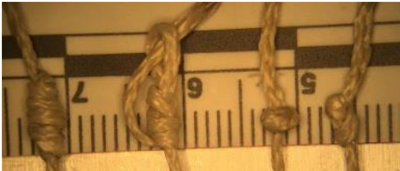
Fig. 9. Knots Tested. From left to right: 8x overhand knot; figure 8 on a bight knot; Ashley stopper knot; Stevedore stopper knot.
