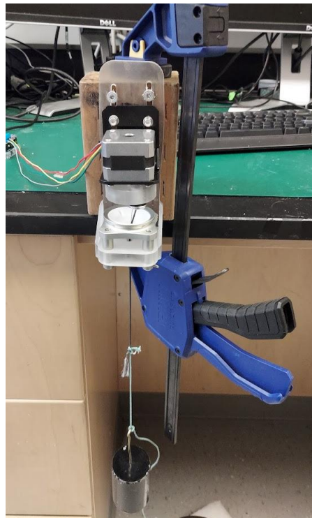
Fig. 10. Tether testing setup. The tether was run through the tether guide, and weights were hung at the bottom. There is a motor at the top of the apparatus that applied rotations to the tether.
