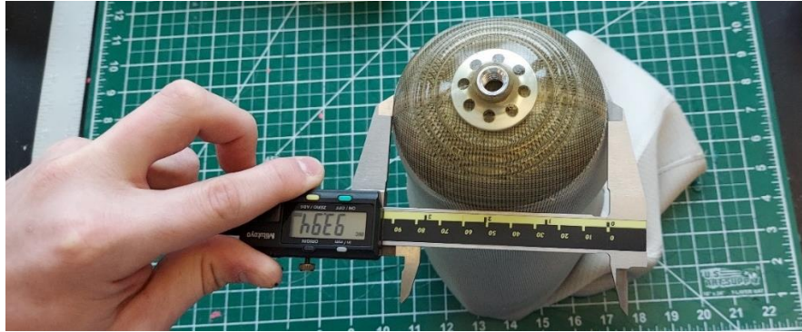
Fig. 5. Measurement of umbrella diameter for use in ferrous liner fabrication.
