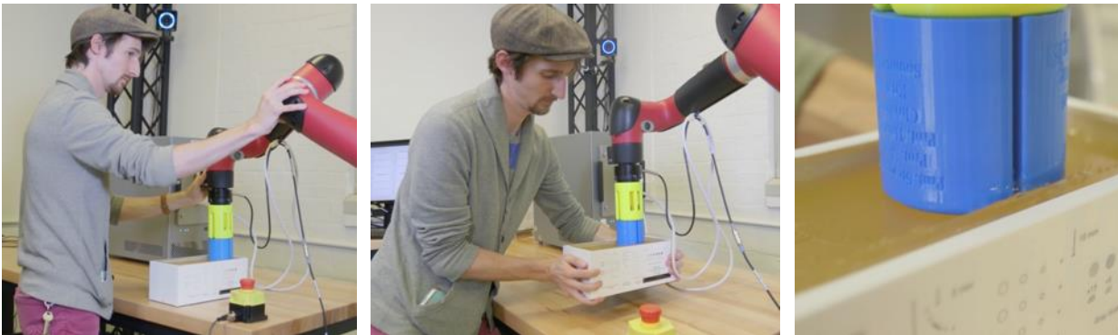
Figure 2: Images showing positioning and experiments with the robotically assisted ultrasound scanning of a tissue phantom.
