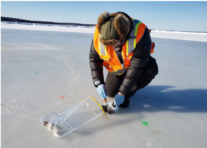
Figure 5. Collecting swept particle piles with a drywall knife and a paint brush.
