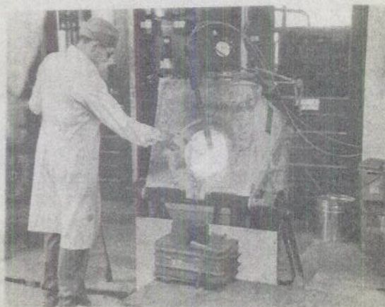
FIG. 34- ADDING FERROMANGANESE TO THE MELT.
