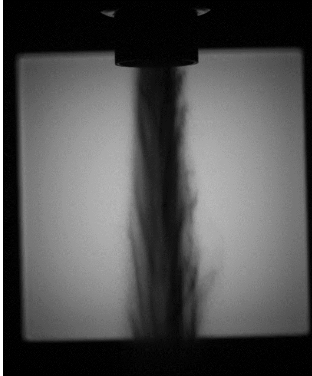
Figure 3-5. Sample unprocessed powder plume image captured with visualization equipment.
