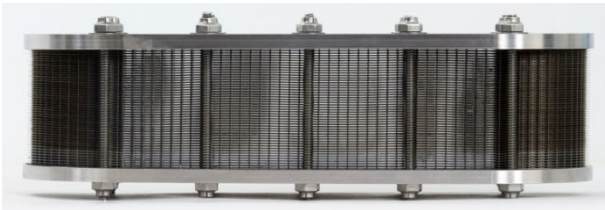
Figure 1. Microchannel Heat Exchanger Produced Using Creare's HAM Technology. Highly uniform array of microchannels enable high surface area density. Efficient coupling of MOF sorbents with process streams yields very rapid kinetics. Module in photo is 9 in. long.
