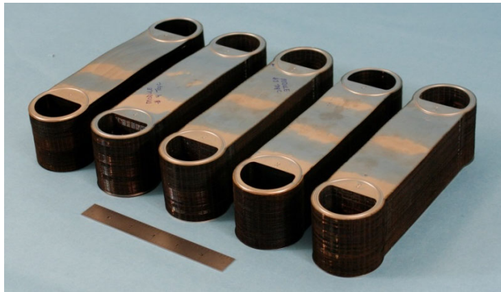
(a) Five 100-Plate Modules From the Recuperator of the Rolls-Royce 700 hp M250 Gas Turbine Engine
