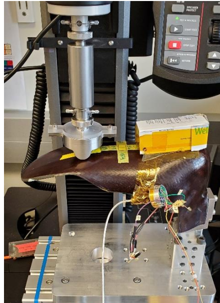
Fig. 12. Test set up for characterizing footplate strain gage sensitivity to ground reaction axial force. A white box with yellow tape is covering the strain gages and wires to minimize the risk of mechanical damage.
