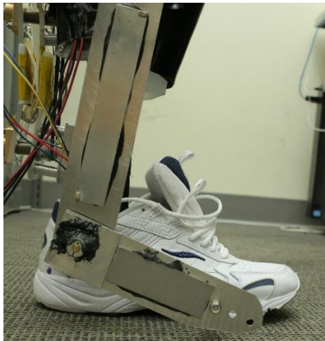
Fig. 2. Independent ankle angle measurement device used to verify bending signal data.
