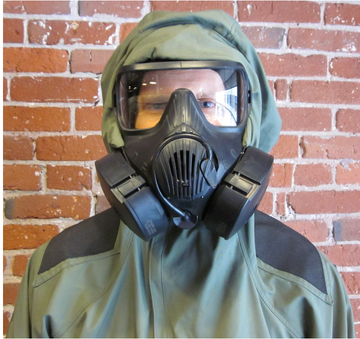
Figure 18. Generation 5 Hood/Mask Interface with JSGPM.
