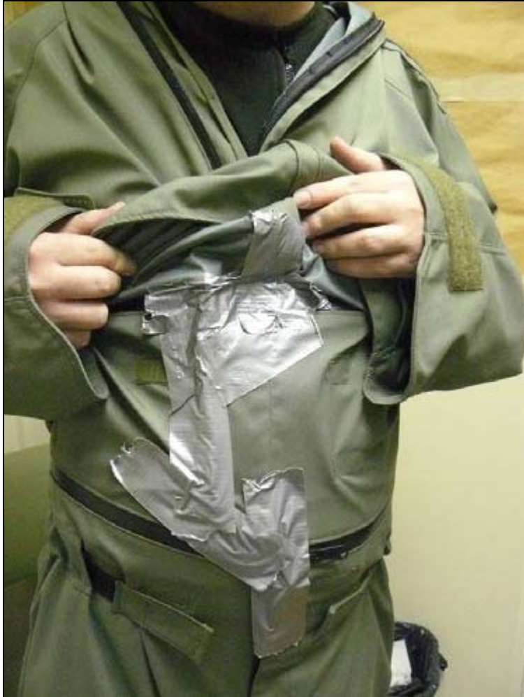
Figure 33. Duct Tape Added to Integration Panel Area before Generation 5 Torso FAST Test 3.
