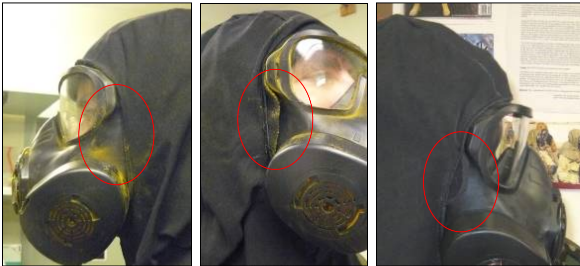
A. Without Modifications. B. With Knitted Insert C. With Neoprene Insert
