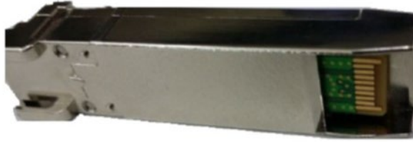
Fig. 4 SFP28 Passive Loop-back Module 4
