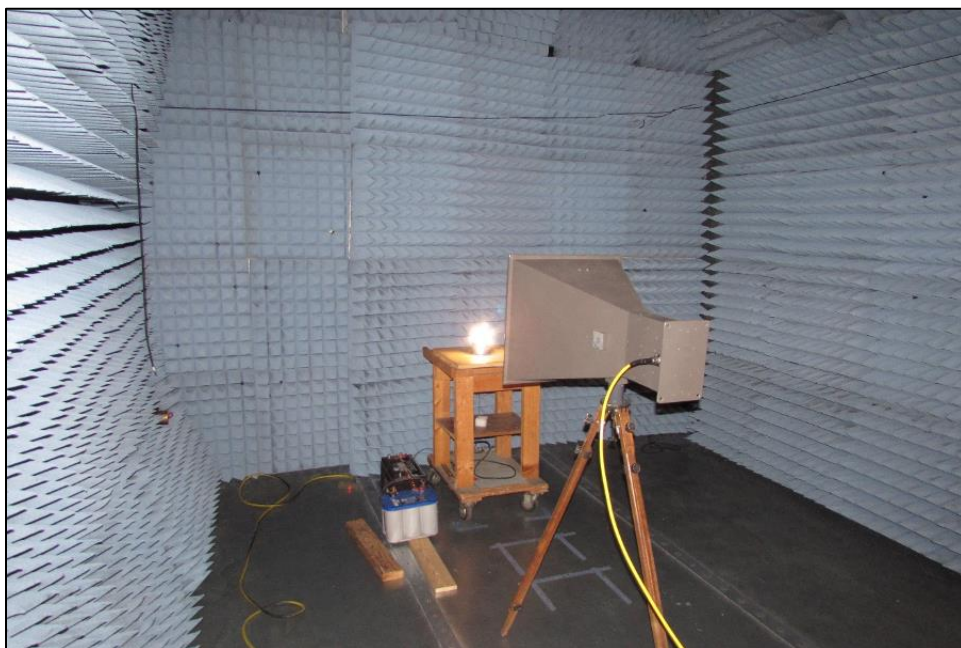
Figure 6. Radiated emissions test setup for L-Band data collection.
