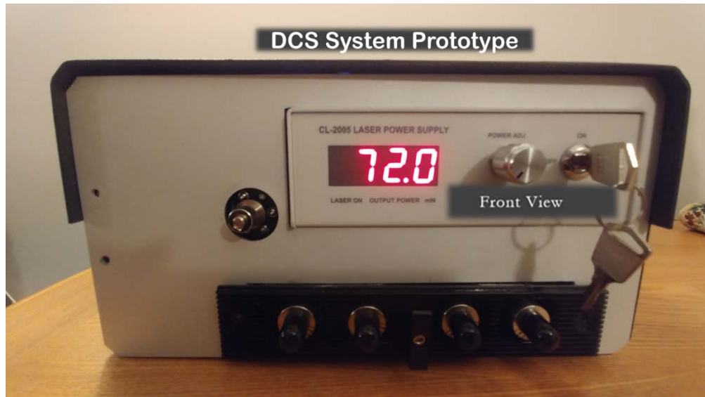
Figure 1. The first prototype of the DCS system. The customized enclosure is designed with the dimensions of: Width x Depth x Height = 10.3”x 11.8” x 5.3”.
