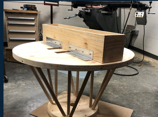
Mounting fixture for a 6x1 tile configuration
