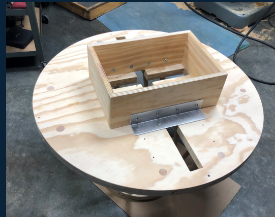
Mounting fixture for a 3x2 tile configuration
