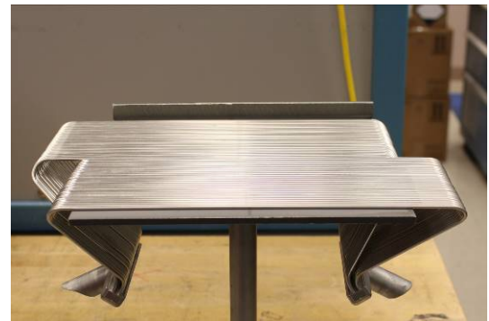
Figure 4. The Gas Tubing Array, note that all sixty tubes have the same shape and length and are divided into two opposite groups of thirty tubes.
