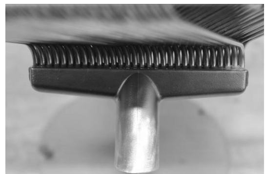
Figure 8. From this orientation it can be seen that the shape of tubes allows the two groups of thirty tubes to align into two rows in the header
