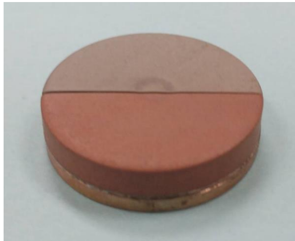
Figure 12. Split, 1-inch diameter ablation target TGT50 (Fe-rich half A at bottom).
