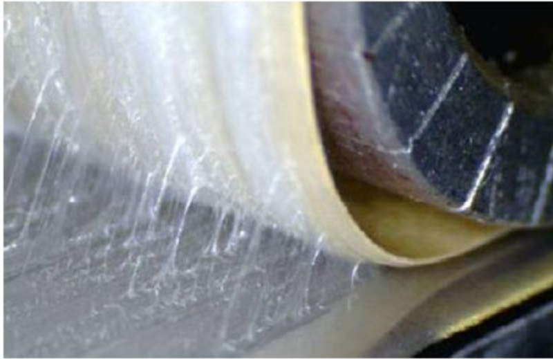
Figure 8. Cohesive failure of prepreg tack and fibrillation [10].
