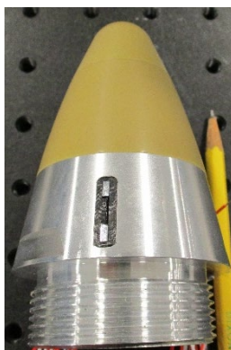
Figure 1 Yawsonde solar sensor assembly placement on a 155-mm fuze
