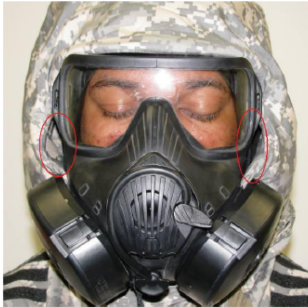
Figure 3-11. Large gaps (circled) at temple areas of hood brim/mask interface. TP1 in 31B shell.
