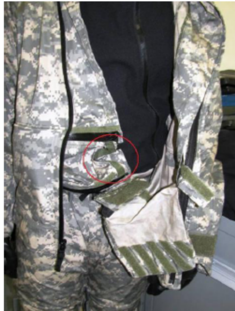
Figure 3-1. TP1 wearing 31B shell, showing Flap B's mating point not laying flat prior to securing waist closure (Flap B mating point circled). All shells exhibited this issue.
