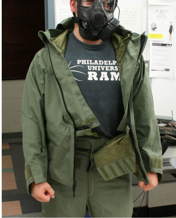
Figure 31. Integration Panel Zipped First to Jacket.
