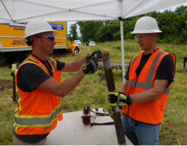
Figure 2.3. Capping and sealing the frozen core section prior to placing on dry ice.
