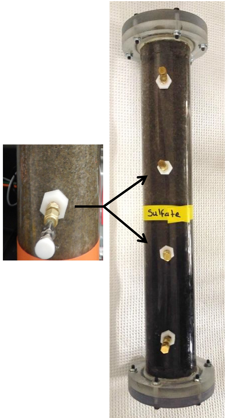
Figure 6.1. Photographs of one of the soil columns used for this project. The insert shows detail of the sample port construction, which is further described in the text.
