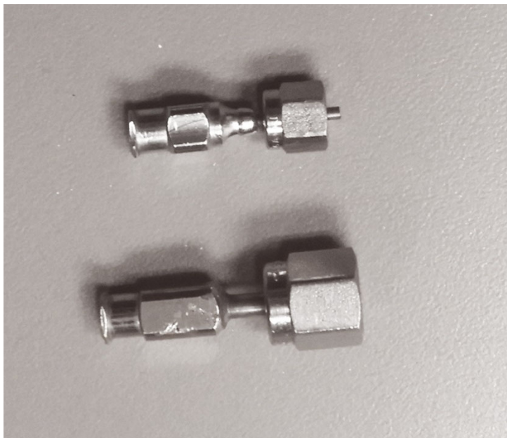
Figure 4.4. Luer to Swagelok adaptors. The 1/8" adaptor uses an 11-gauge needle, the 1/16" adaptor uses a 16 gauge needle.
