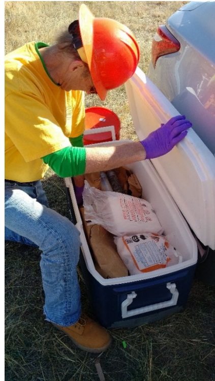
Figure 2.4. Packing frozen soil cores and dry ice into coolers for overnight shipment.
