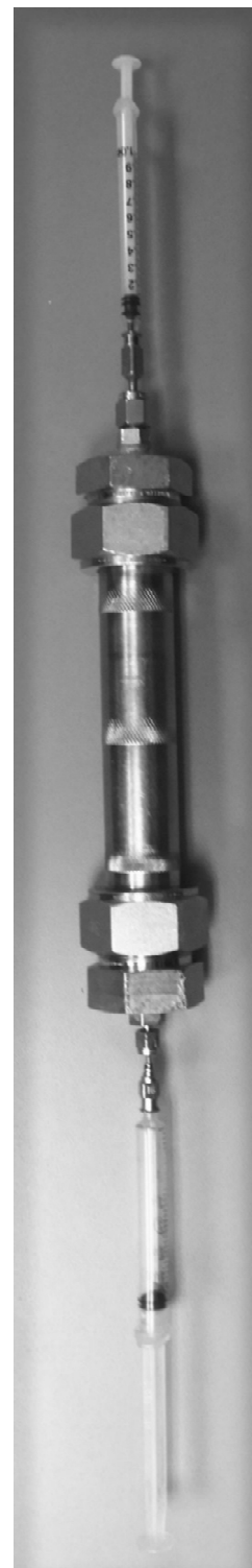
Figure 4.6. RTR with upper and lower syringes attached. (Process for injecting analytes and for sampling)
