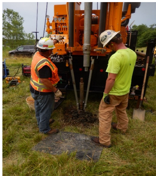
Figure 2.1. Photograph of the hollow-stem auger used for most of the core sampling (Here at Indian Head, MD).
