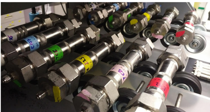
Figure 4.5. Rolling Tube Reactors (RTR) reactors used for the kinetic studies. Here they are shown on the roller system that rotated them at ~6 revolutions per minute.
