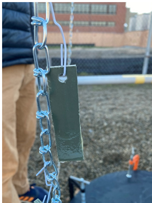
Figure 53. Biological indicator (biofilm-laden fiberglass coupon) attached to chain which was suspended into tank
