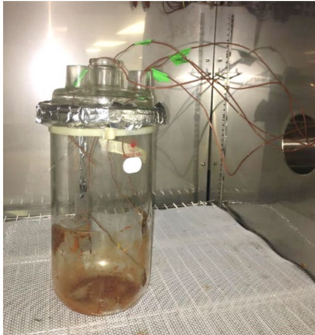
Figure A-4. Empty 3-L contaminated vessel being treated with passive HAD inside an environmental chamber (note: thermocouples were placed inside the vessel with one suspended in air and the other touching the interior wall of the vessel).
