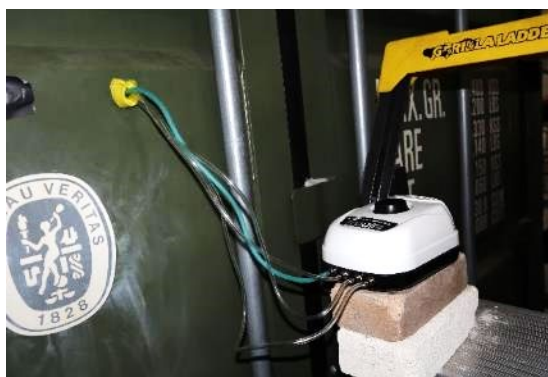
(D) Air pump placed outside the shipping container and connected via silicon tubing to the air diffusers placed inside the column unit.
