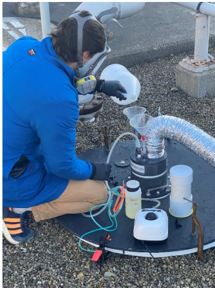
Figure 54. Chemical precursor being added to GDU to initiate ClO 2 generation
