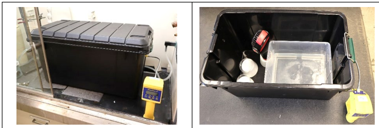
Figure 10. Tote ClO 2 gas treatment test system used for bench-scale ClO 2 efficacy testing
