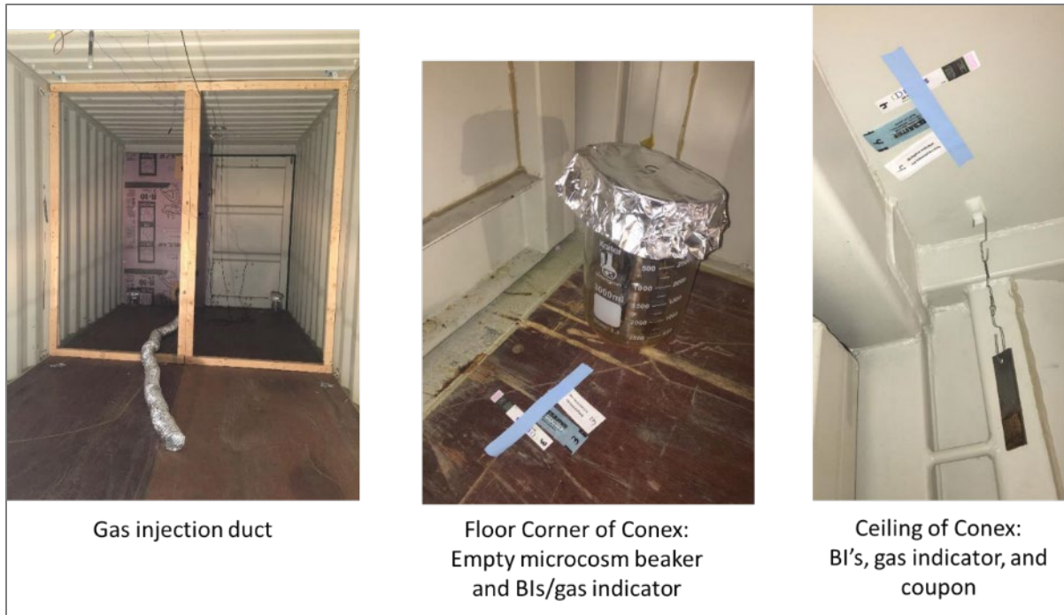
Figure 39. Interior of shipping container (i.e., full-scale test system) showing location of microcosm vessels, BIs, and gas indicator strips
