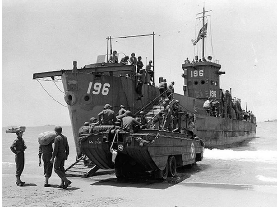
Figure 2. Landing Craft, Infantry and DUKW. USS Landing Craft Infantry National Association, "LCI Facts," accessed 25 February 2020, http://usslci.org/facts/ .
