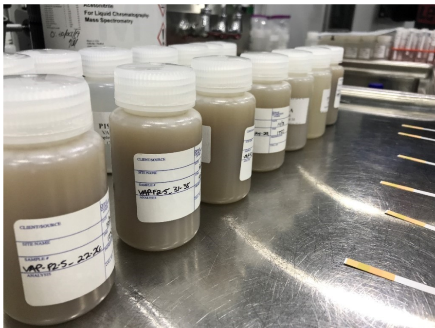
Figure 6-1. Typical Sediment in Groundwater Samples
