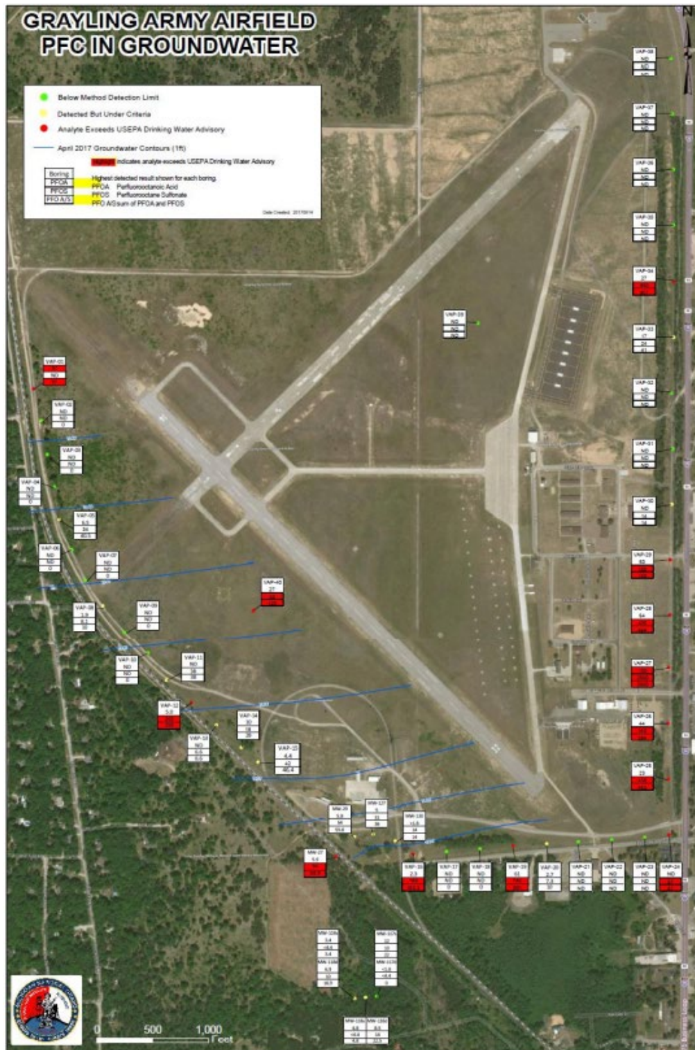
Figure 4-2. GAAF Perimeter Groundwater Sampling Results
