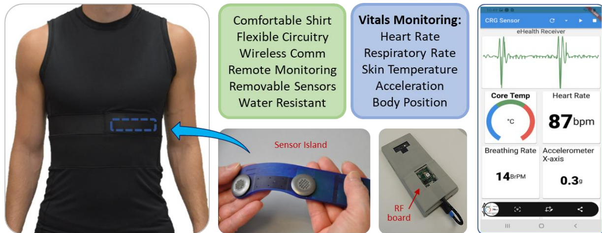
Figure 2: Phase II Prototype eHealth Garment with Sensor Island and Mobile Phone with App
