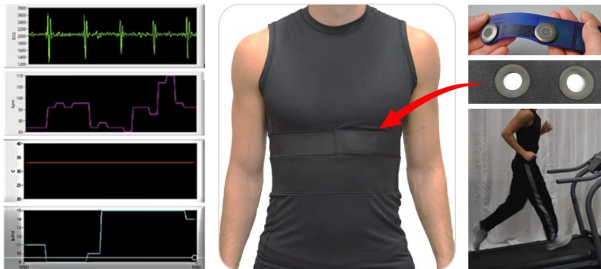
Figure 3: Prototype eHealth Garment Sensor System and example testing
