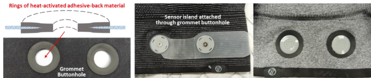
Figure 10: Examples of initial grommet-like buttonholes for dry electrode integration
