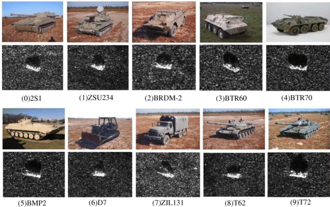
Figure 2.1: Examples of MSTAR targets and photographs of the targets. MSTAR images contain target, background, and shadow information. Figure adapted from [83]
