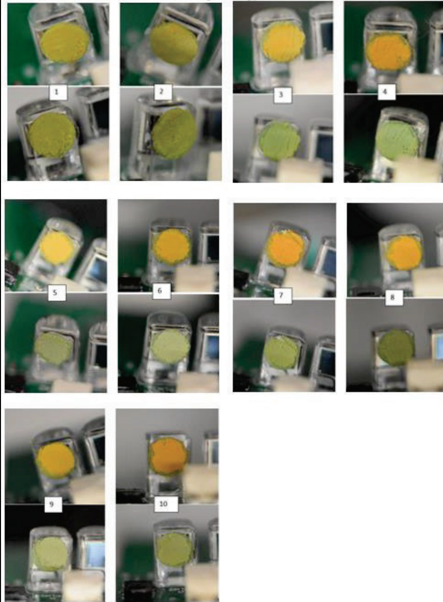
Figure 30. Dots before (top) and after (bottom) HD exposure for 1–10 trial runs at 0.335–1.78 mg/m 3 range in concentration. Five-day-old dots were used in trials 1 and 2.
