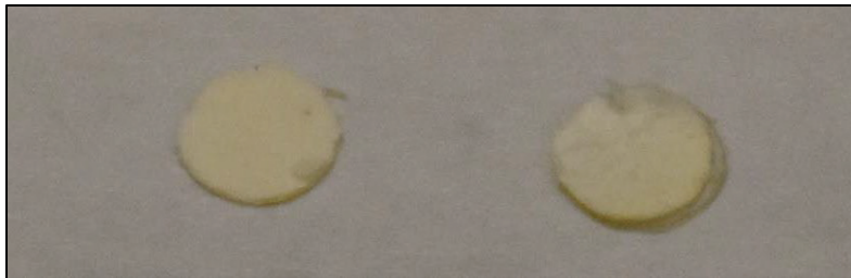
Figure 39. Dots before (left) and after (right) VX exposure for concentration run 2.
