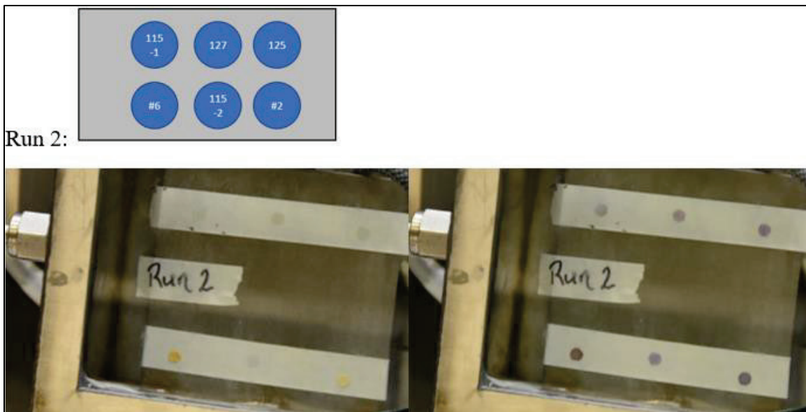
Figure 14. Run 2: (Top) Second of three randomized arrays of six dots. (Bottom) Images of dots in chamber before (left) and after (right) GB exposure. GB exposure was 20.1 \text{ mg/m}^3 for 20 min for six randomly placed dots.
