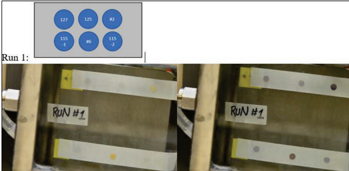
Figure 13. Run 1: (Top) First of three randomized arrays of six dots. (Bottom) Images of dots in chamber before (left) and after (right) GB exposure. GB exposure was 16.4 \text{ mg/m}^3 for 20 min for six randomly placed dots.
