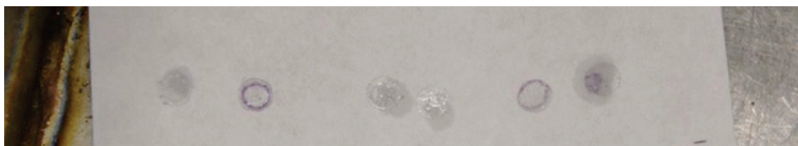
Figure 11. Exposure of 0.2 \mu\text{L} of neat GB to the same old and new G115 dots as shown in Figure 10. Dots were left in a sealed glass jar over the weekend.
