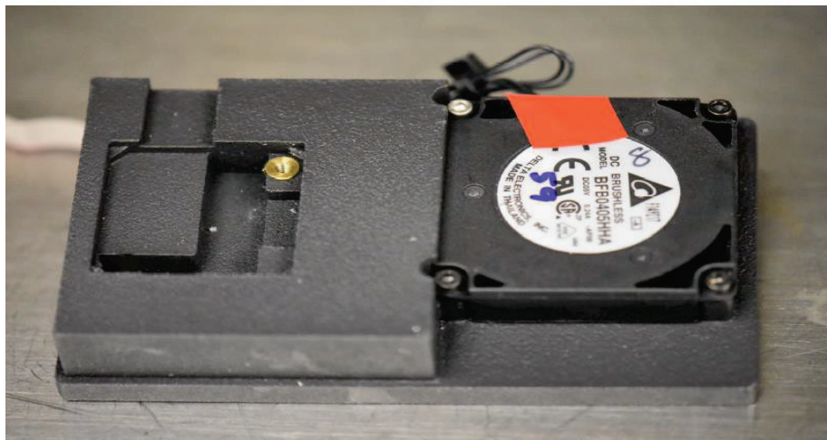
Figure 3. Back of MOSA GEN1 blower fan housing. Fan (right) and slot where optical sensor is installed once dot is attached (left) are shown.
