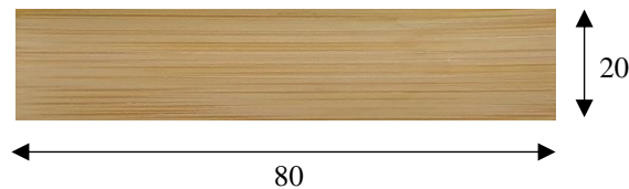
Figure 2. Dimensions of a Bamboo panel.
