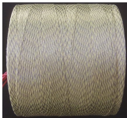
Fig. 14—Completed tether winding
