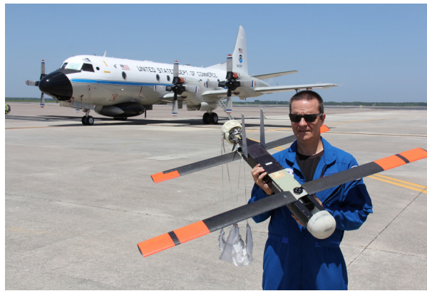
Figure 7. Coyote employed for hurricane research; launched from the P-3 in the background [32] (Figure courtesy of NOAA).
