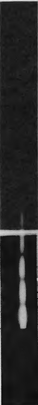
COPPER SPARK IN AIR \frac{1}{4} " DIAM. CU. RODS, \frac{3}{32} " SEPARATION
