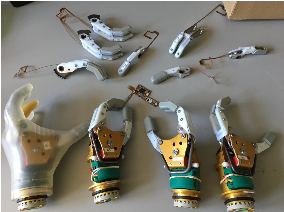
Final hands (with cosmeses removed) that were ultimately sent to subjects, plus spare parts retained for any necessary repairs.
