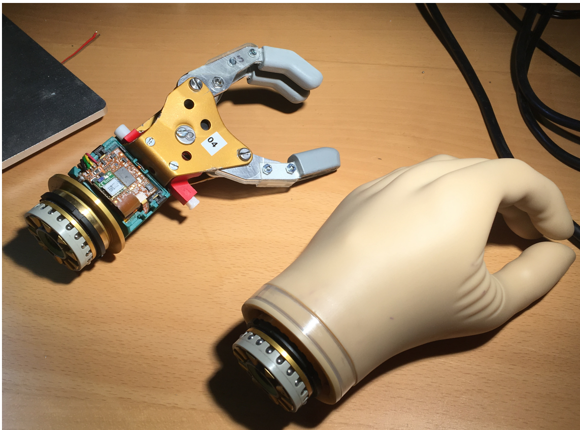
Left: fully assembled prosthetic hand showing custom electronics (with protective cover removed), sensors, cable covers and wiring. Right: A second fully assembled prosthetic hand with the cosmesis installed.
