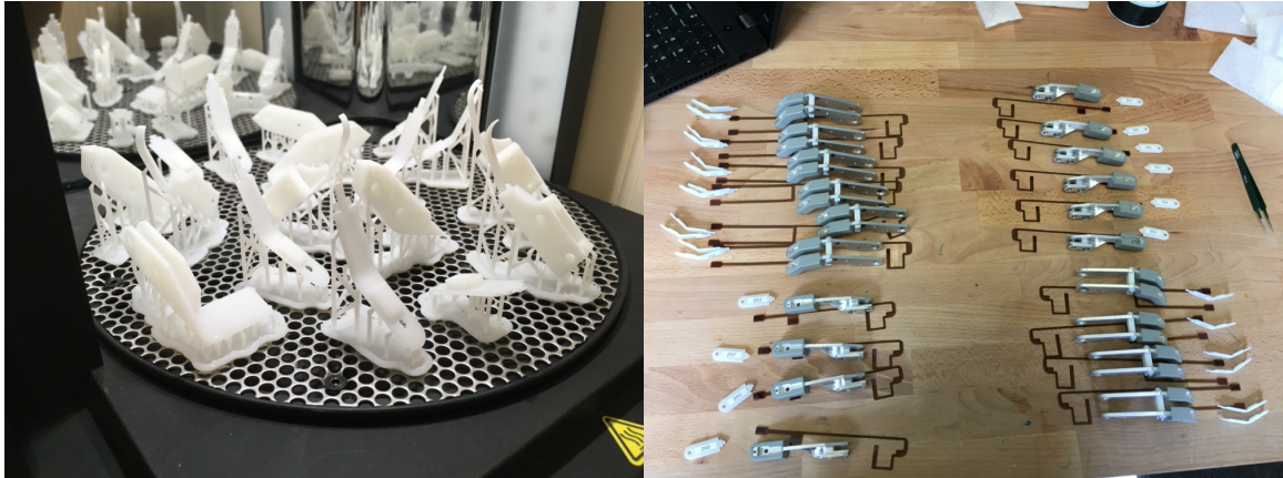
3D printed parts of improved finger covers (left) and final assembly of left/right fingers and thumbs (right)
