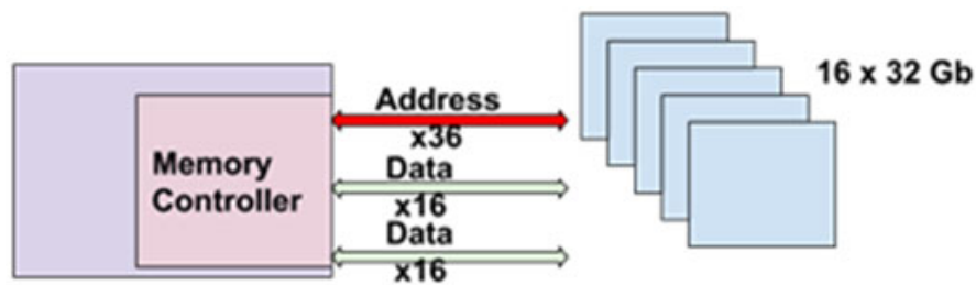
Figure 4. Memory design using 16 x 4 GB DRAM chips
