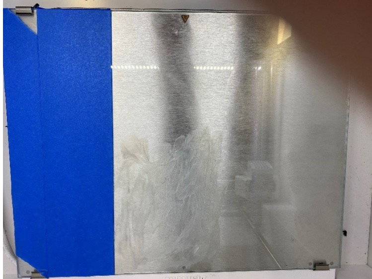
Figure 15: Bed Adhesion Test (Left: Blue Painter's Tape, Middle: Glue, Right: Bare Glass)
