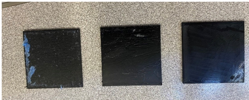
Figure 16: Printed Protopasta Samples on Each Different Adhesion Types (Left: Blue Painters Tape, Middle: Glue, Right: Bare Glass)
