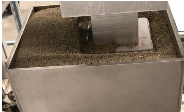
Figure 11: Snapshot of the unconfined shear test showing the shear plate and soil box.
