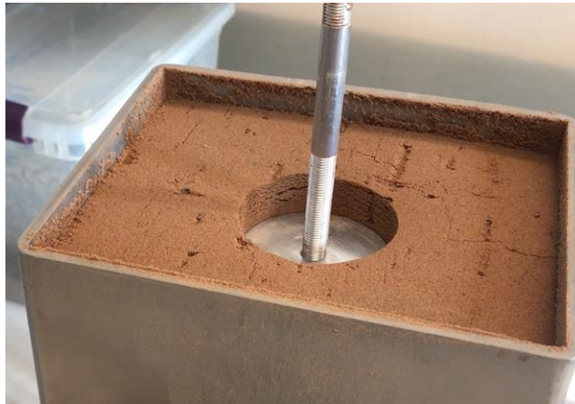
Figure 19: Snapshot of a typical disk penetrometer test.
