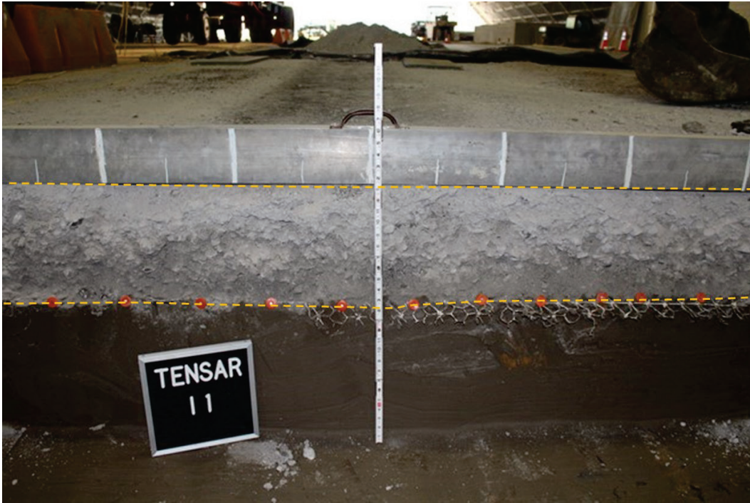
Figure 41. Item 1 (NX950) posttest excavation.
