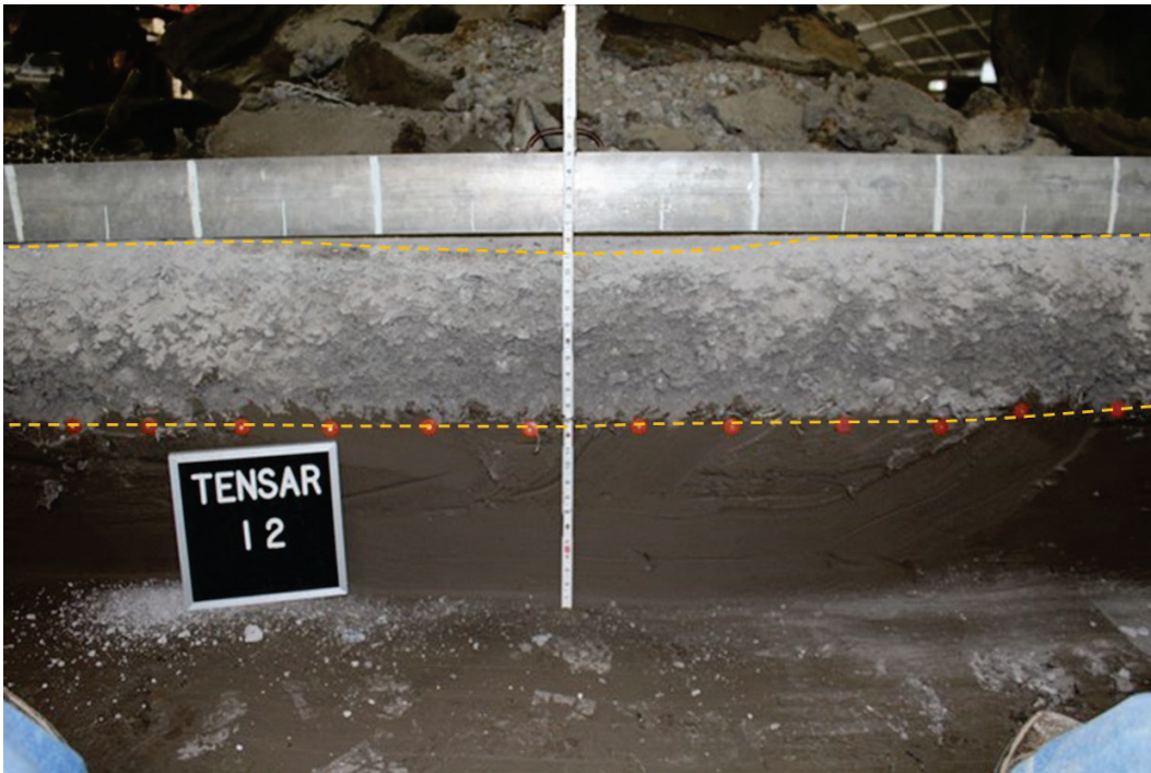
Figure 42. Item 2 (NX750) posttest excavation.
